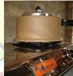
Alluminium cooker with clay casing and base electroplated
