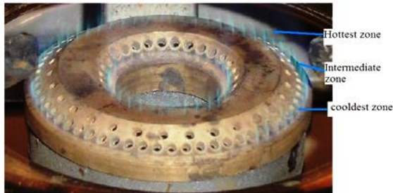
Fig.1 Flame showing zones
